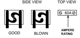
Maxi-fuse cartridges have a transparent colored plastic housing. To check a maxi-fuse cartridge, look at the fuse element through the side of the housing.
