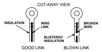
Fusible links are short lengths of wire that are smaller in diameter than the wires they are protecting. Fusible link wire is covered with a special thick, non-flammable insulation. An overload condition causes the insulation to blister. If the overload condition continues, the wire link will melt. To check a fusible link, look for blistered insulation. If the insulation is okay, pull lightly on the wire; If the fusible link stretches, the wire has melted.
