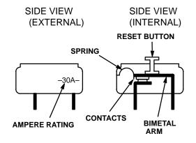
Two types of non-cycling circuit breakers are used; one is reset by removing power from the circuit, and the other is reset by depressing a reset button.
