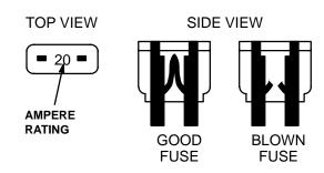
Blade type fuses have a transparent plastic housing. To check a fuse, pull it from the fuse panel and look at the fuse element through the housing. Always replace a blown fuse with a new fuse that has the same ampere rating.
