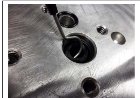
Figure 19 Removing the seal
