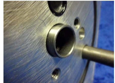
Figure 22 Insert metal spacer over new seal
