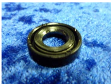
Figure 20 Side of seal to face out toward pump
