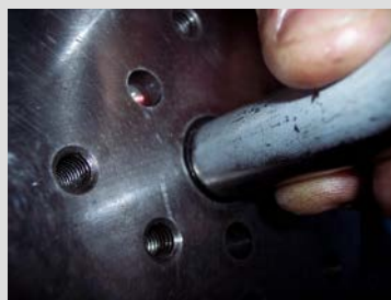
Figure 10 Setting seal in place
