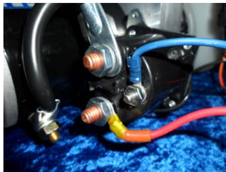
Figure 10 Motor solenoid wiring
