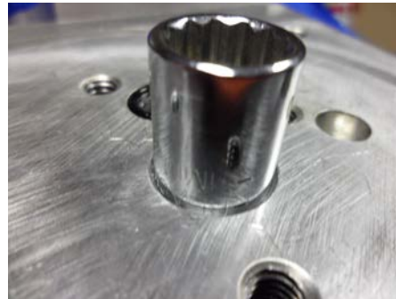
Figure 21 Tap seal into place using upside down socket
