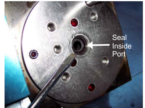
Figure 7 Seal from pump side port hole
